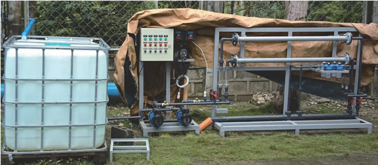
HydroChem Plus Experiment Facility for Anti-scaling
