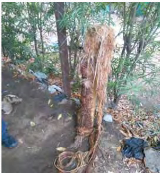
Blockage of water pipelines with trees roots
